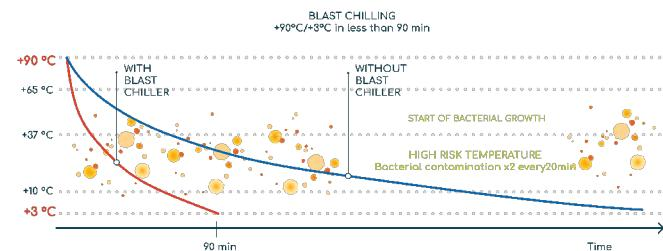
The speed with which the rapid freezing process takes place is essential to achieve micro-crystallisation of the water particles contained in the product. Compared to macro-crystallisation, this allows:
